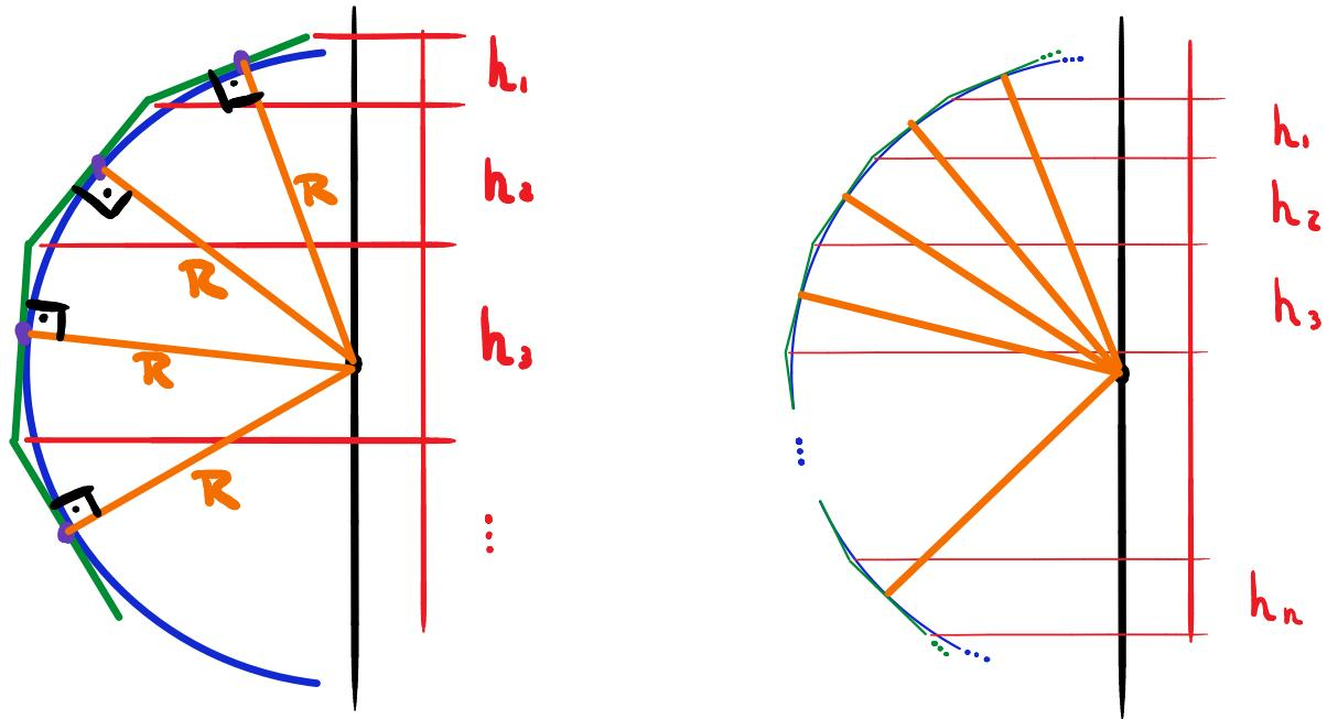
$$\begin{aligned} A_c &= A_1 + A_2 + A_3 + \dots + A_n \\ &= 2\pi Rh_1 + 2\pi Rh_2 + 2\pi Rh_3 + \dots + 2\pi Rh_n \\ &= 2\pi R(h_1 + h_2 + h_3 + \dots + h_n) \end{aligned}$$
